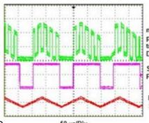
modulated, pulsed and triggered Diode current
